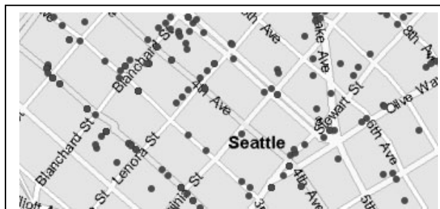
Figure 1: WiFi density in urban centers is such that multiple access points are within range of many locations. Each AP beacons a unique identifier that, along with a mapping database, can be used to lookup a coarse grain position. In this image each dot is an estimate of the position of a WiFi AP in downtown Seattle mapped in a single “wardrive.”
