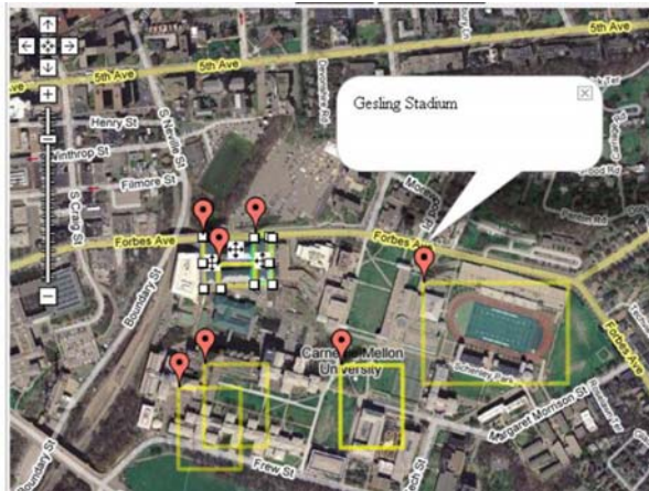
Fig. 4 Defining locations as combinations of rectangular areas for use in location-sensitive privacy rules.
