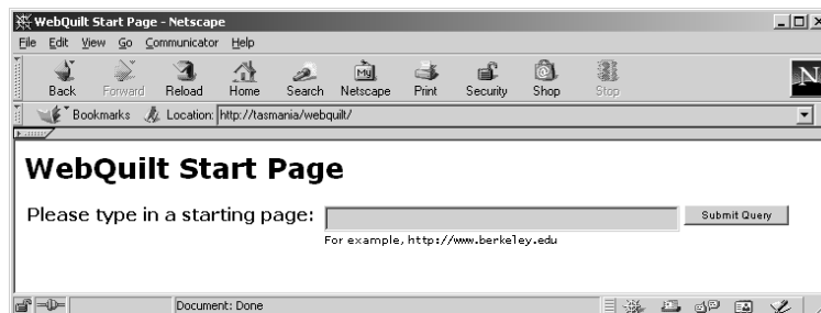
Figure 5. Default page for the WebQuilt proxy. The proxy will retrieve and dynamically modify the URL that is entered.
